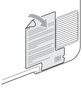
C Connect the telephone line cord. Connect one end of the telephone line cord to the jack on the machine marked **LINE** and the other end to a modular wall jack.
